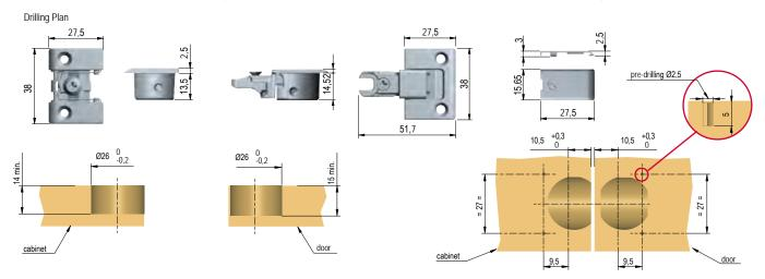
INSTALLATION ON THE CABINET (MINIMUM THICKNESS 18 MM)
