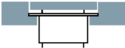
OPTION C Rebated for custom top (12mm max.) in 30mm or greater material.
