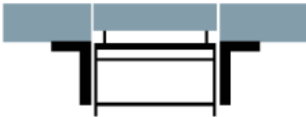
OPTION D Under-mounted for custom top (12mm max.) in 20mm material ONLY. *requires an undermount kit replacing standard collar*
